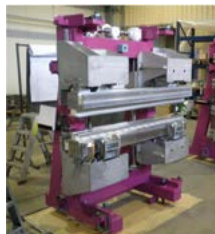
Revolver Mobile Undulator Carriage for the E.S.R.F. in France. Repeating Parallelism tolerance between the beams is 0,05 mm over 2,5 meters, incl. beam rotation.
