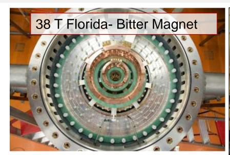
Electrical Power: 22 MW (40 kA, 550 V) Water cooled: 160 l/s Limited by mechanical stress
