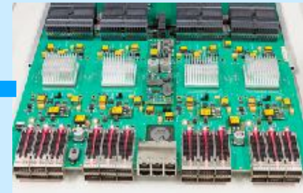
UniBoard2 FPGA Processing Platform • Data throughput: 3 Tera bit per second (Tbps) • Processing capability: 5 Tera MAC/s
