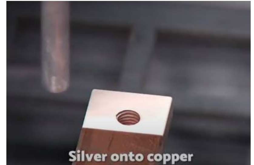
Silver on Copper Bus Bar – electro-plating replacement
